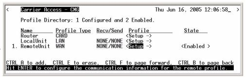
Profile Directory Window The Remote Profile Window will change as options are selected. The graphic below displays the window as NAT Gateway is enabled.
